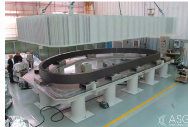
Figure 20 WP introduction into Vacuum chamber for testing
