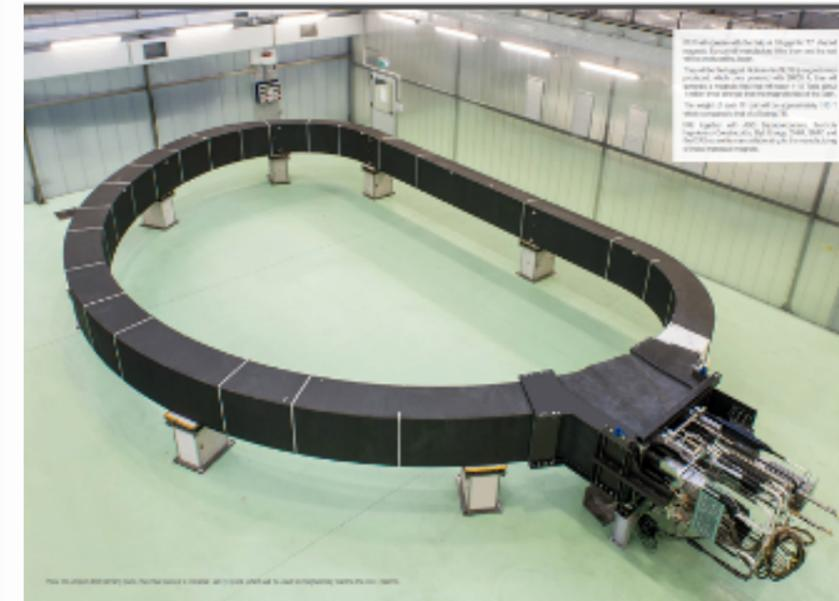
Figure 11. View of a WP inside the dedicated alpha-magnetic clean area at ASG premises (La Spezia). White tape visible on the coated surface was used to visualize the location of the sections to be measured and simplify the preliminary alignment of the device.
