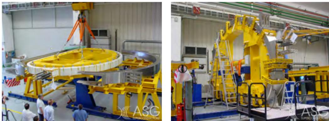
Figure 21, 22 WP and coil casing onto the assembly tooling / Assembly tilted in vertical position for welding execution
