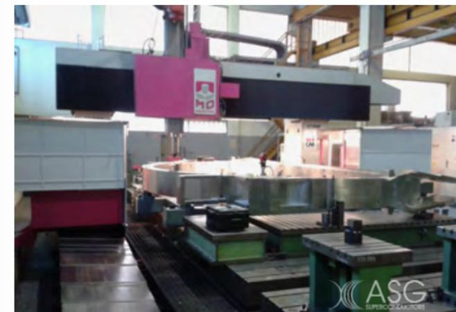
Figure 24 TFC interface machining (courtesy of Officine CLP)
