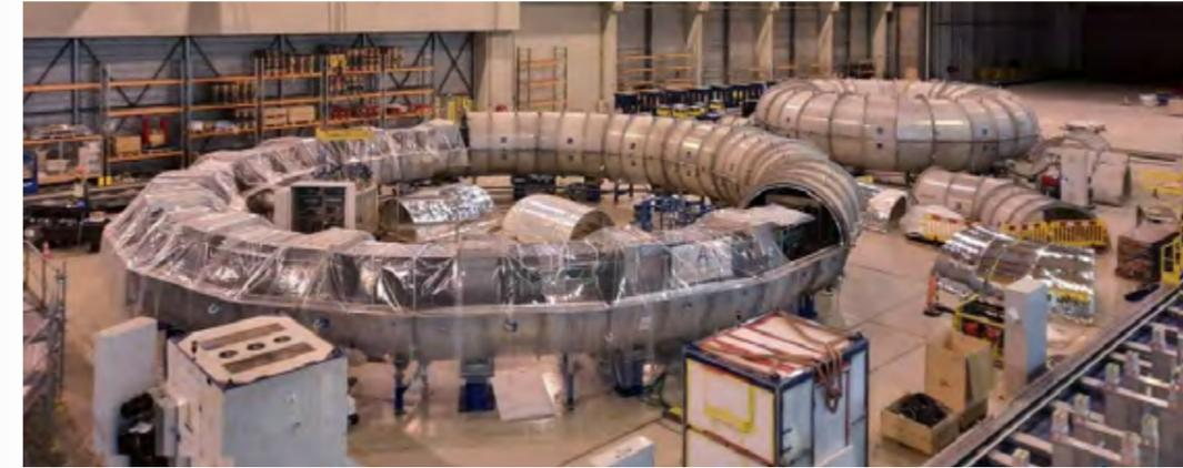
**Figure 2** The dedicated area for the cryostats: On the right, the smaller cryostat is assembled and cold testing of the PF6 coil is in progress. On the left, the medium sized cryostat is about to be assembled for the final cold test of PF5.
