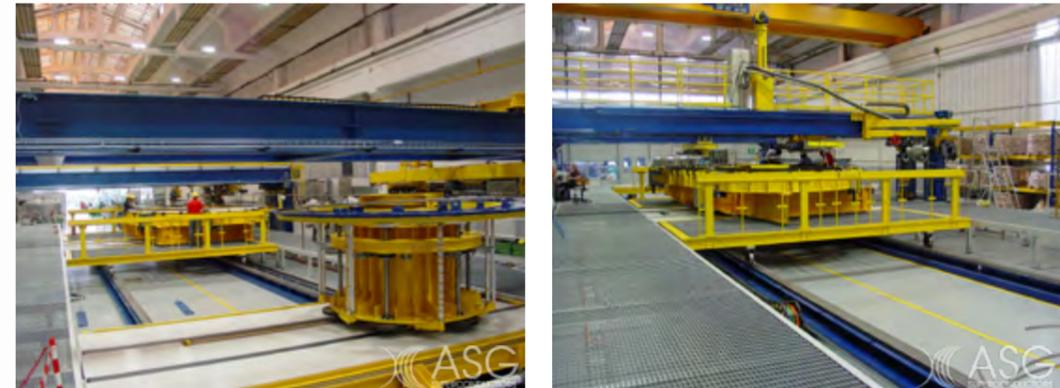
Figure 11, 12 Winding Line-Unwinding spool / Winding Line-Winding Table
