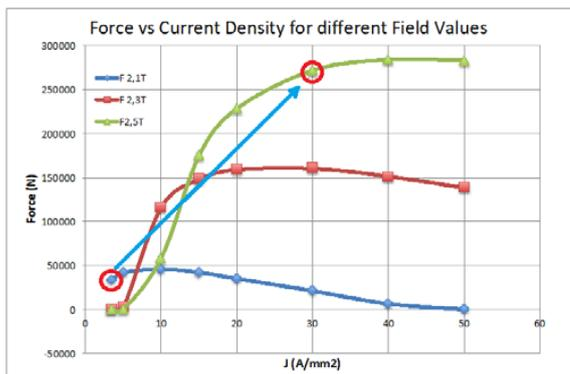
**Figure 7** Force vs Current Density for 3 values of B. For a normal conductor, working above 3-4 A/mm<sup>2</sup> is not possible (the best option is the blue curve). For a superconducting machine it is possible to achieve 30 A/mm<sup>2</sup>, jumping to the green curve.
