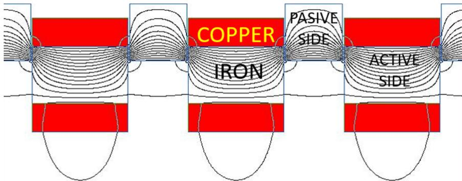
**Figure 6** A Switched Reluctance Machine has an Active side (copper and iron pole) and a Passive side (iron) moving one respect of the other.
