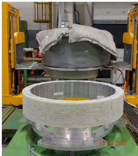
Figure 5. Shrink-fitting operation at ASG premises
